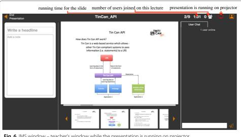
Fig. 6 IMS window – teacher's window while the presentation is running on projector
