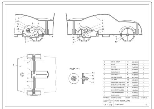
**Fig. 1** Example of a technical drawing from a graphic project (reproduced with the student's permission). The product selected is a toy car powered by a friction motor
