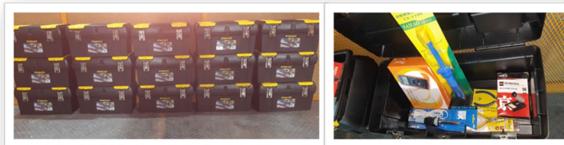
Fig. 7 The figure shows the kit with its box, which contains: two resistors, four capacitors, three motors, five LEDs, two solar cells, a multimeter, soldering iron, desoldering pump, soldering cable, tip and cutting pliers, a rubber gun, and cables. The kits were given to the students to make the robots in their homes
