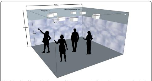
**Fig. 1** Overview of four-wall CAVE set-up used in the present study. Eight projectors presented the virtual environment on the walls. Tracking cameras visible in the corners were used for positional tracking, enabling embodied interaction
